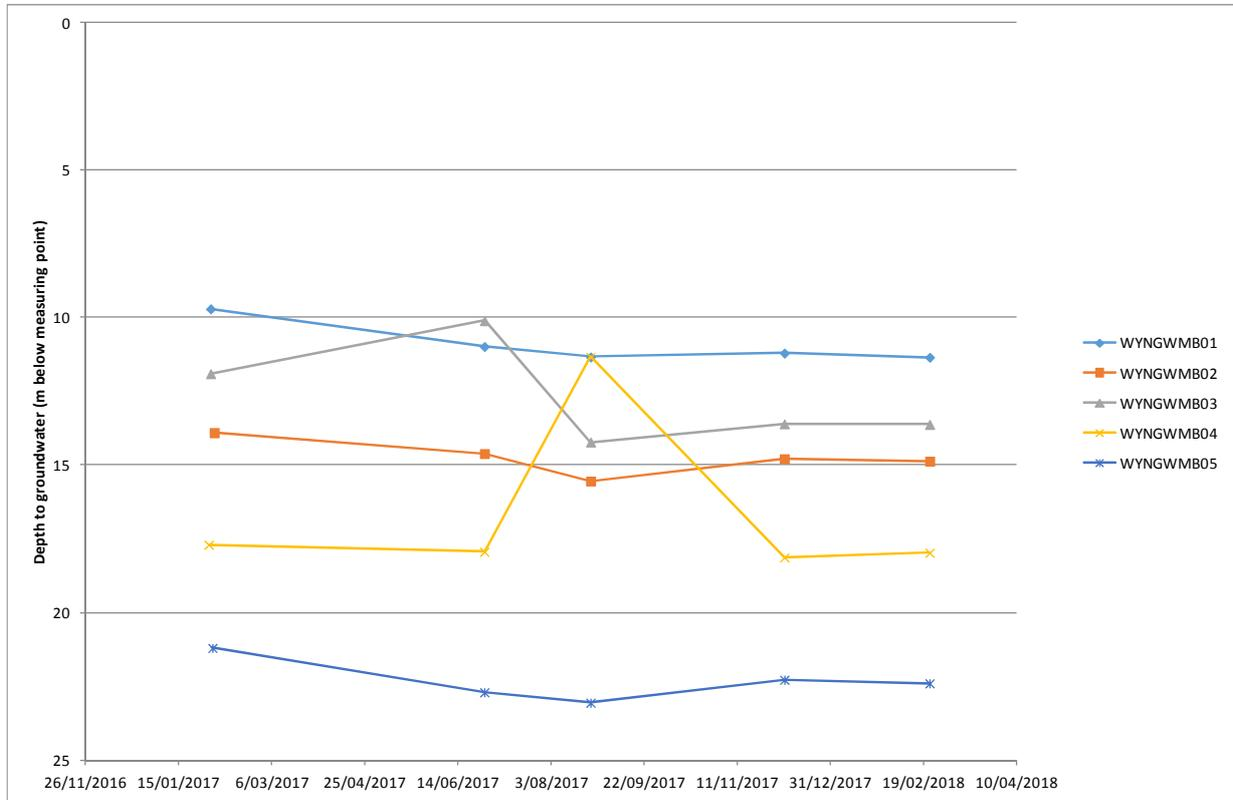
**Figure 2: Chart of depth to groundwater in Wynberg deposit groundwater monitoring bores**
